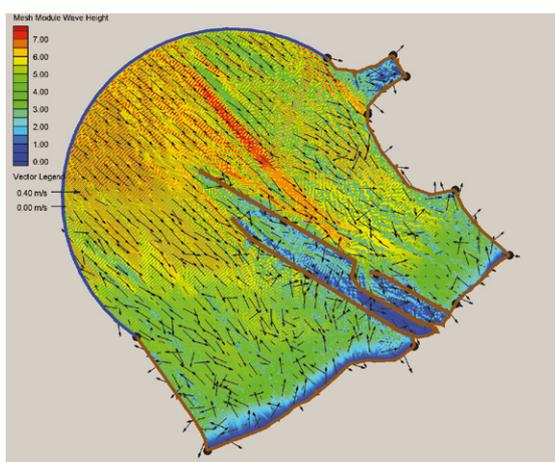
*Wave pattern around and within the channels, based on the actual incident waves, used for the armouring design of the inner breakwater slopes*
